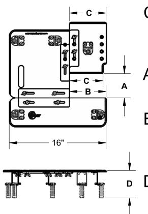
ADJUSTS TO 5-1/2" OR 6" LONG ON THE BACK OF THE FREEARM OR SEWING BED BY REVERSING THE BACK ADJUSTER
